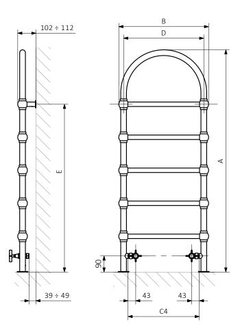
$A-Height \quad B-Width \quad C1-C5-Distance \ between \ pipe \ centres \quad D-Horizontal \ distance \ between \ mounting \ bracket \ centres \\ E-Vertical \ distance \ between \ mounting \ brackets \quad F-Distance \ between \ a \ mounting \ bracket \ and \ the \ bottom \ of \ the \ radiator$
