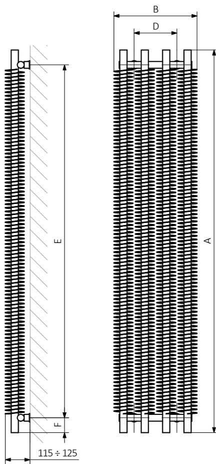
A — Height B — Width C1-C5 — Distance between pipe centres D — Horizontal distance between mounting bracket centres
